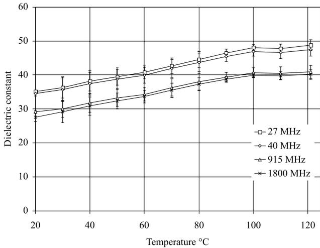
Fig. 5. Dielectric constant of cooked macaroni noodles as a function of temperature at four frequencies.
