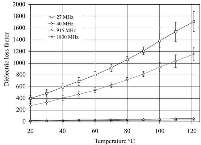
Fig. 7. Dielectric factors of macaroni and cheese as a function of temperature at four frequencies.
