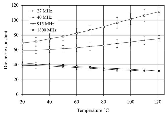
Fig. 4. Dielectric constants of cheese sauce as a function of temperature at four frequencies.
