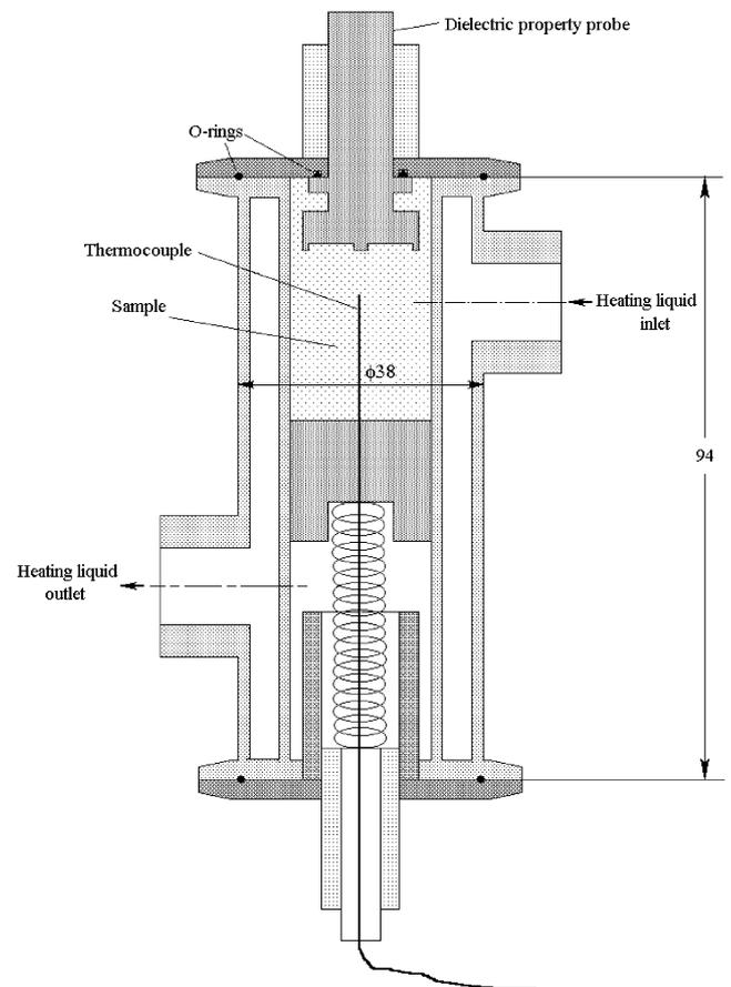
Fig. 1. Diagram of pressure-proof dielectric test cell (stainless steel), dimensions in mm.
