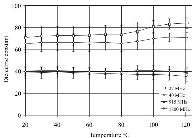
Fig. 3. Dielectric constants of macaroni and cheese as a function of temperature at four frequencies.
