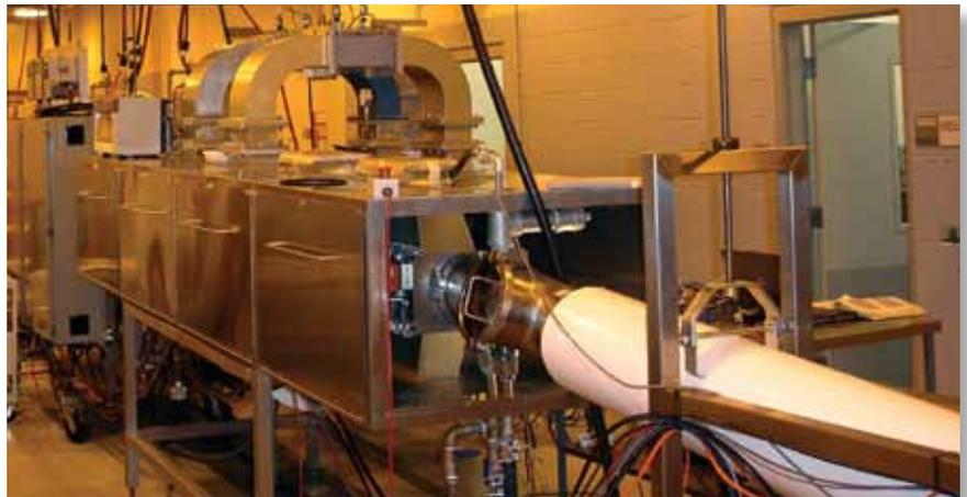
*Second-generation microwave sterilization system at Washington State University.*
