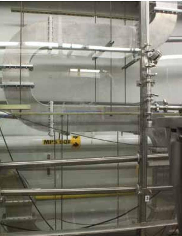
Segment of the *Ultraseptics continuous flow microwave sterilization* installation at North Carolina State University pilot plant.
