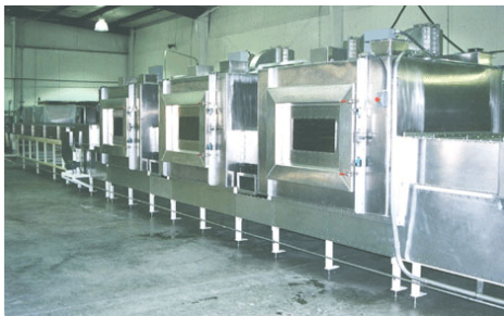
A 300 kW MW oven with conveyor for continuous heating and drying applications.
